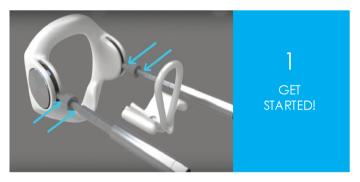
Before fastening the plastic front piece, make sure there is 1mm (0.04 inch) of space on both sides of the handle on the adjustment screw, facing both the hexagonal piston, as well as the base plastic ring. This enables the adjustment screw to expand on both sides of the handle.
